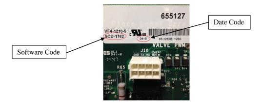
Production of furnaces with the new logic control board began the first week of March; furnaces produced with date code of W1C5 and later contain the new board. Source 1 inventory has also been stocked with the new control boards; boards shipped as of the date of this letter contain the new logic.
